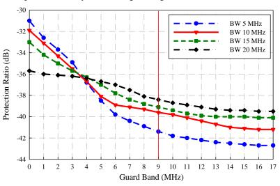
Fig. 3. Protection ratios for DTT interfered by LTE-UL for different LTE BW.
