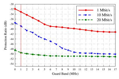
Fig. 2. Protection ratios for DTT interfered by LTE-UL with a bandwidth of 10 MHz, for different traffic loadings.
