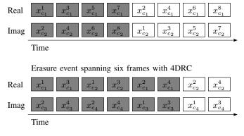
Fig. 2. Interleaving of components with inter-frame interleaving across eight frames.
