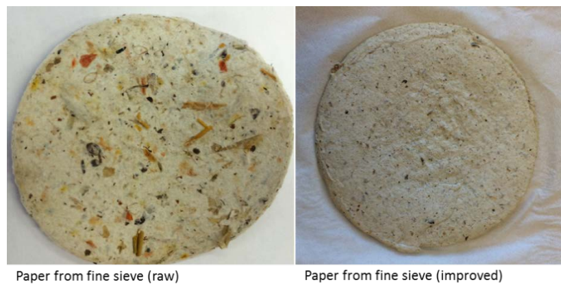
Figure 4. Result for different sieving techniques to retain cellulose from waste water
