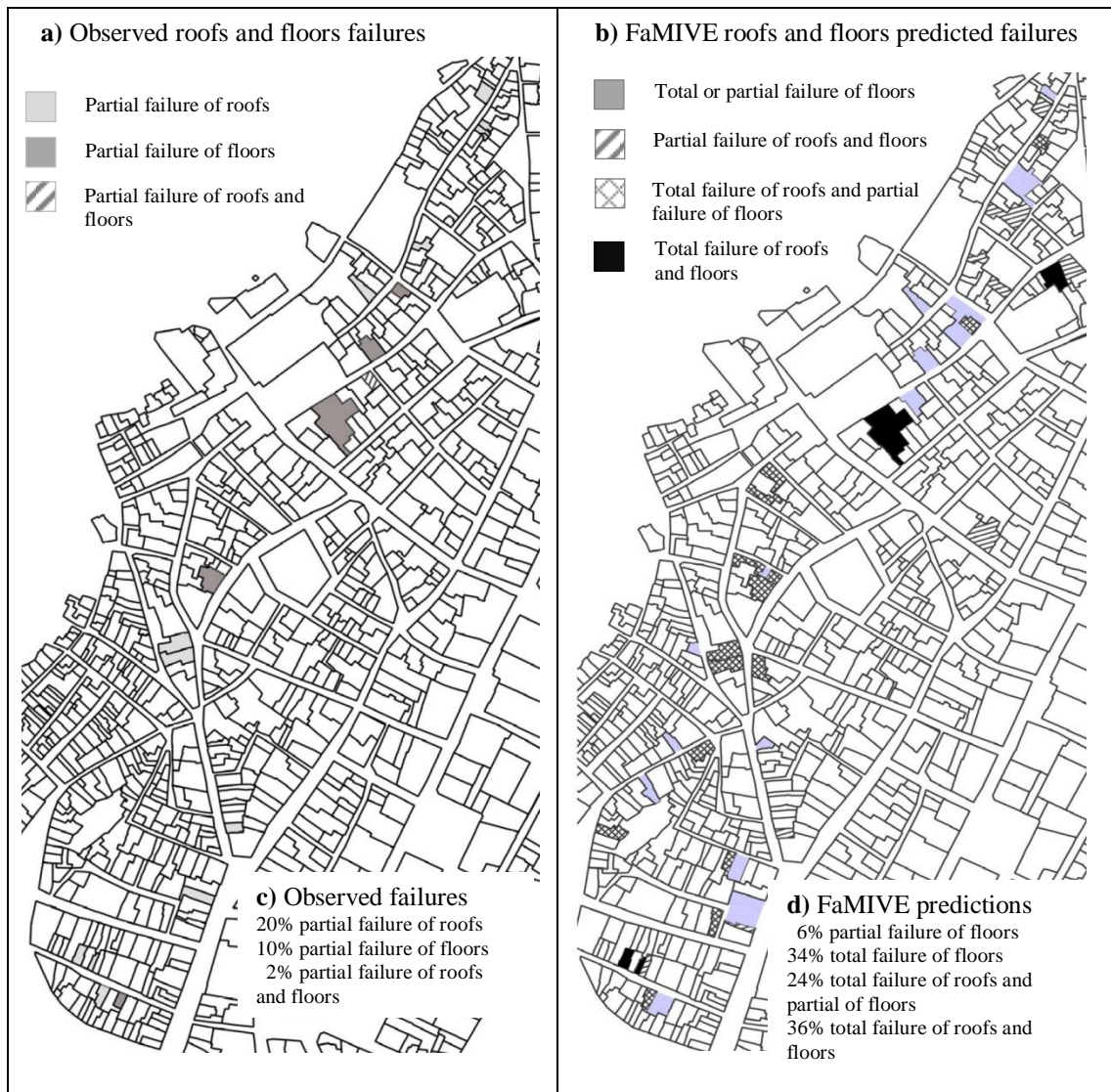
Fig. 18 Observed and predicted roofs and floors failures
