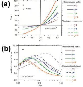
20 Fig. 9 (a) Calculated *I-V* and (b) rectification ratio vs. KCl concentration curves for asymmetrical pores obtained from single U ion tracks (continuous lines) and from the equivalent conical pores (dotted lines). The curves are parametric in the etching time.
