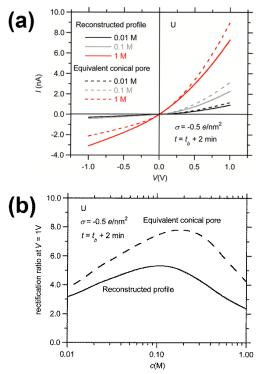
60 Fig. 8 (a) Calculated *I-V* and (b) rectification ratio vs. KCl concentration curves for asymmetrical pores etched for 2 minutes after breakthrough from single U ion tracks (continuous lines) and equivalent conical pores with the same surface charge concentration, pore base radius, and electrical conductance at 100 mV (dotted lines). The curves are parametric in the KCl concentration.
