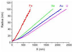
**Fig. 6** Reconstructed tip profiles,  $r_x(x)$  of asymmetrical pores etched for 2 minutes after breakthrough, where x is the distance from the tip. The profiles are obtained for single U, Au, Xe and Fe ion tracks.
