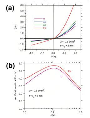
**Fig. 7** (a) Calculated *I-V* and (b) rectification ratio vs. KCl concentration of curves for asymmetrical pores etched for 2 minutes after breakthrough. Profiles are obtained from single U, Au, Xe and Fe ion tracks.
