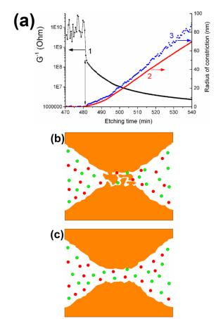
Fig. 3 (a) Conductometric etching of a single Fe ion track. The electrical resistance G-1 (1) and the constriction radius, calculated by both the double-cone (2) and the two funnel (3) models, as functions of etching time. (b) Simplified sketch of a pore with a residual part of the electroconductive latent track in the middle. (c) Open pore after breakthrough.
