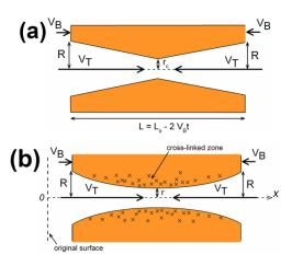
Fig. 2 Two models for two-sided ion track etching: a) double-cone, b) quasi-doubly-conical pore consisting of two funnel-like halves symmetrical to each other with respect to the central plane. The cross-linked zone around the track core is marked with crosses. For other designations, see the text.
