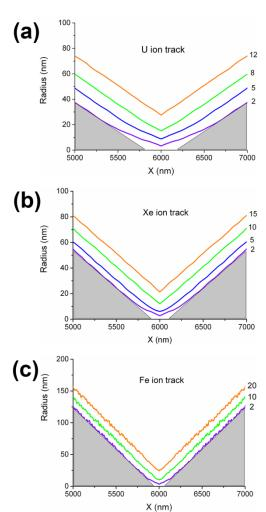
65 Fig. 4 Central part of reconstructed pore profiles of the U (a), Xe (b) and Fe (c) ion tracks, etched from both sides. Center plane: x = 6000 nm. The numbers at the curves denote the etching time after breakthrough, in minutes. Inscribed triangles are intended to show the deviation from double-cone geometry.
