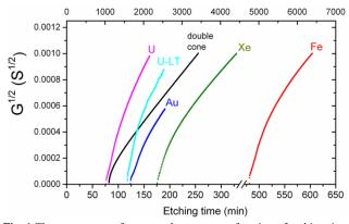
30 Fig. 1 The square root of pore conductance as a function of etching time (scale at bottom), for single tracks of U, Au, Xe and Fe ions in PET foil. The theoretical curve calculated by eqn. (3) is shown for comparison. Etching conditions: 9 M NaOH; temperature: 22°C (U, Xe) and 18°C (Au, Fe). The curve marked U-LT was measured at a temperature of 35 0.5°C and normalized to the specific conductivity at 22°C (time scale at top).
