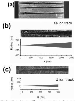
Fig. 5 Confirmation of pore profiles using scanning electron microscopy.
