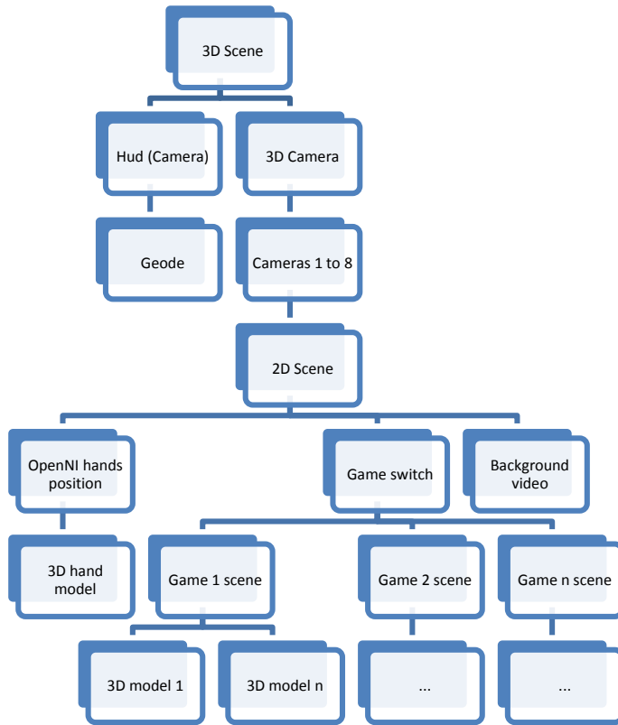
Figure 4.3: OSG graph scene used to create the 3D scene integrating OpenNI with a 3D layer specific for the autostereoscopic display
