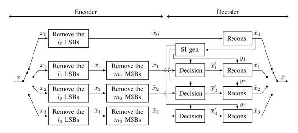
Fig. 1. Block diagram of the GPCM coding of an image block.
