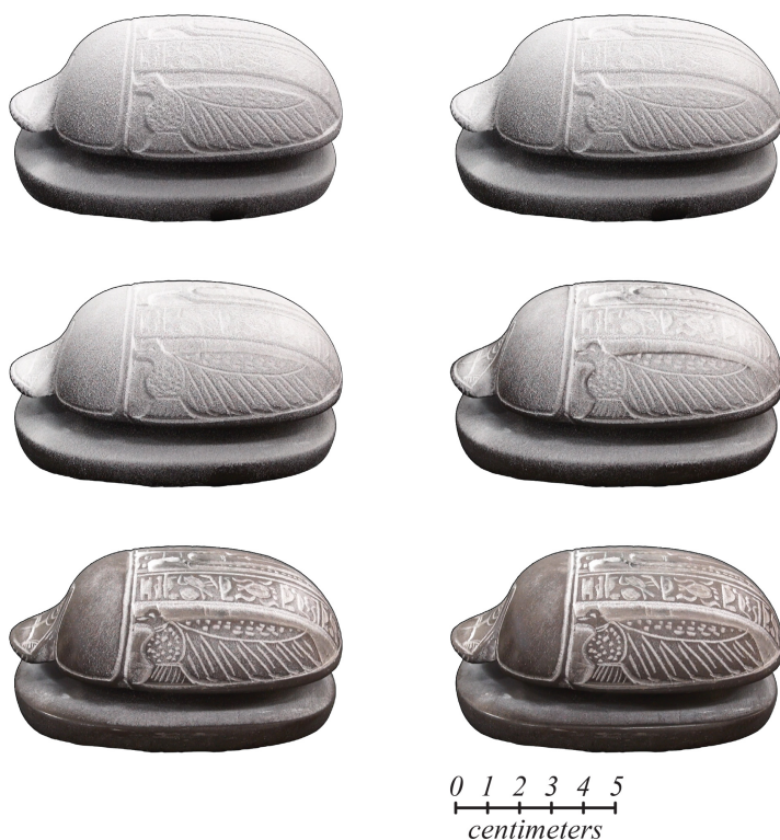
Figure 4.2: From left to right and top to bottom, the sublimation of cyclododecane applied on an artifact. Images are captured in 45 seconds intervals since the application of the spray (top-left picture). The process has been accelerated pointing a hair dryer towards the object.
