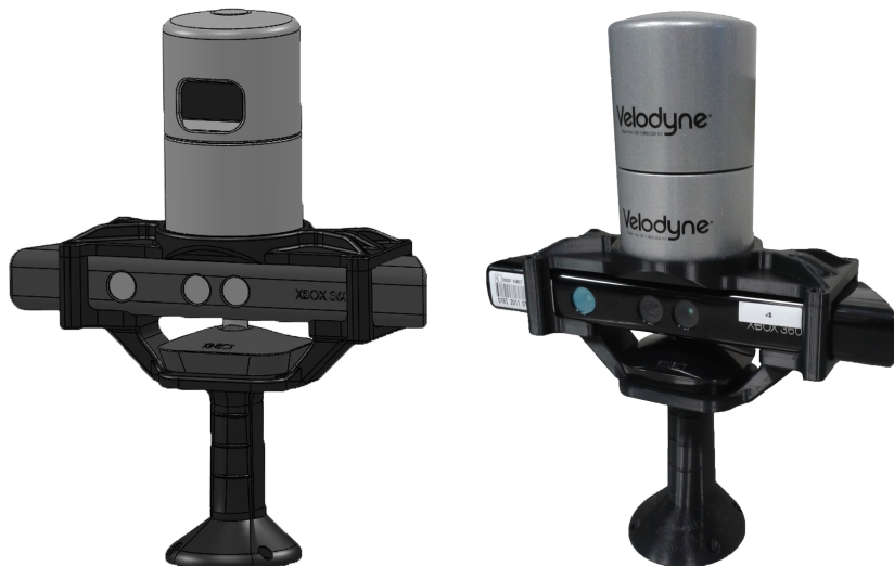
Figure 7.30: Design of the sensor holder used for generating training datasets. (left) 3D model of the holder. (right) 3D printed version with both sensors attached.
