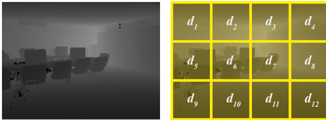
Figure 7.16: Proposed Kinect descriptor. (left) A synthetic range map computed by the GPU using the ground truth point cloud. (right) Proposed criteria for computing the descriptor: each square is the set of values used to compute each median distance ( d_i ).
