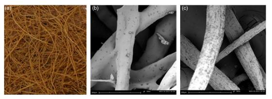
FIGURE 1. a) Detail of coconut fibers. b) Photograph of the fiber without fireproof treatment taken using an electron microscopic. c) Idem with fireproof treatment.
