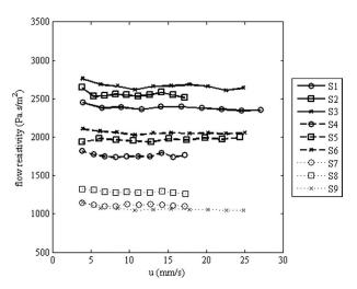
FIGURE 4. Flow resistivity obtained for different air flow rates. S1, S2 and S3 correspond to samples of coconut fiber without fireproof treatment 2 cm thick, S4, S5 and S6 correspond to samples of coconut fiber without fireproof treatment 3 cm thick, S7, S8 and S9 correspond to samples of coconut fiber without fireproof treatment 4 cm thick.
