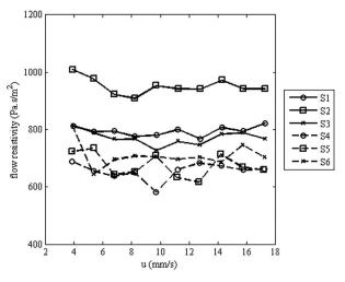
FIGURE 5. Flow resistivity obtained for different air flow rates using samples with fireproof treatment. S1, S2 and S3 correspond to samples 2 cm thick, and S4, S5 and S6 to samples 3 cm thick.
