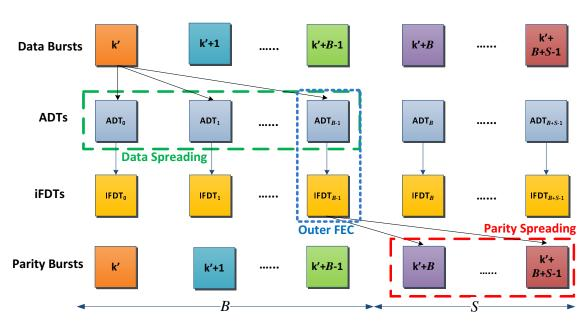
Fig. 2. Inter-burst interleaving with BB-iFEC with the parity transmitted after the data (D = 0). The interleaving depth in number of interleaved bursts M, is equal to the data spreading factor, B, plus the parity spreading factor, S. After the generation of a parity burst, the data and parity spreading windows are shifted one element.
