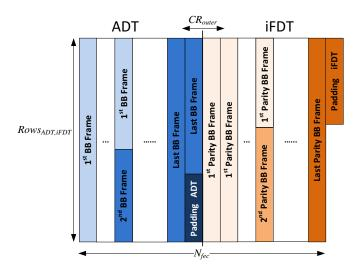
Fig. 4. BB-iFEC encoding matrix. ADT (Application Data Table) and iFDT (iFEC Data Table). The padding bits of the ADT are not transmitted. The padding bits of the iFDT can be used to transmit in-band L1 signalling.
