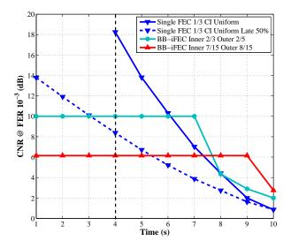
Fig. 9. Performance comparison between single FEC and BB-iFEC for an overall code rate CR 1/3 in the TU6 channel at 10 Hz Doppler. Modulation is QPSK.
