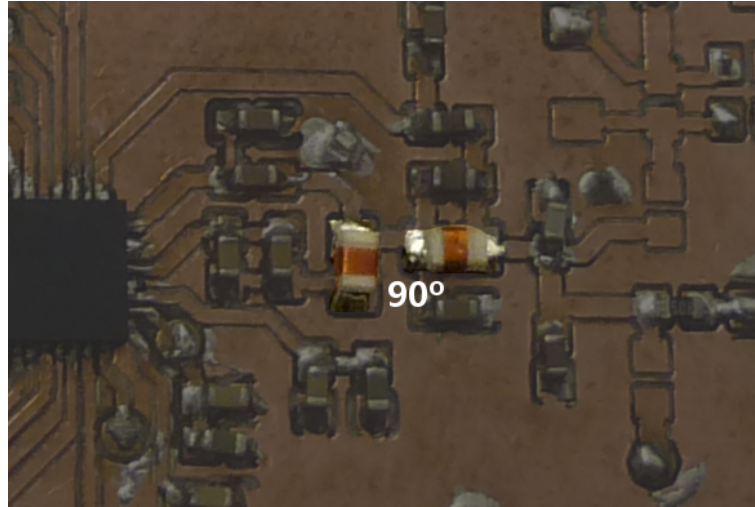
Figure 5.12: Pair of inductors at 90^\circ orientations with respect to each other
