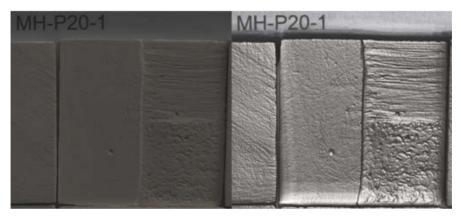
Fig. 9. A test sample of texturized bone filling is seen under an oblique light angle (left) and with RTI specular enhancement (right).
