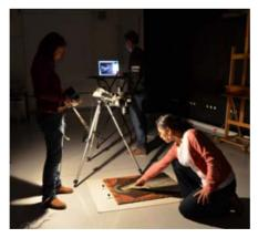
**Fig. 2.** Conservators during data capture using the RTI Highlight method, where a light source is moved around the object and a new image is taken for each light angle.
