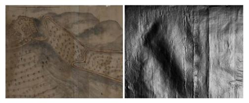
Fig. 3. Watercolor detail visualized in RTI with flat light (left), and specular enhancement (right). When the color values are reduced and reflectance increased, it is possible to see the faint outlines on the road and rectangular structures (upper left area). Deformations, wrinkling, joints, and fold marks are also enhanced through specular filters.
