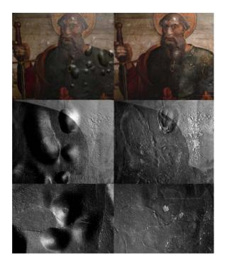
Fig. 8. Three details of panel painting "San Pablo" surface, visualized with RTI before (left column) and after (right column) blisters were consolidated and flattened.
