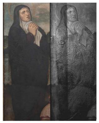
Fig. 5. Detail panel painting "El Calvario", visualized in RTI with flat light (left) and specular enhancement (right). RTI offers a clearer and more detailed view of the wood support deformation, and the cracking, scratching, losses, and cupping of pictorial layers.
