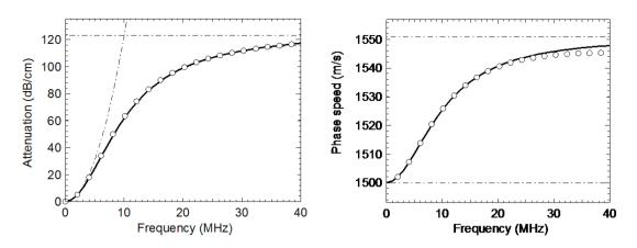
Fig. 1 Left: Attenuation retrieved by the numerical method (circles), theoretical (continuous line), low frequency limit ( $\omega^2$ ) and high frequency limit  $\omega^0$  (dashed line). Right: Dispersion retrieved by the numerical method (circles), theoretical (continuous line), low frequency limit ( $c_0$ ) and high frequency limit ( $c_\infty$ ).
