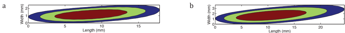
Fig. 4. Focus aberration comparison in the films for an incidence angle of 10° in 2D (a) and 3D (b) models for a layer thickness of 2.7 mm
