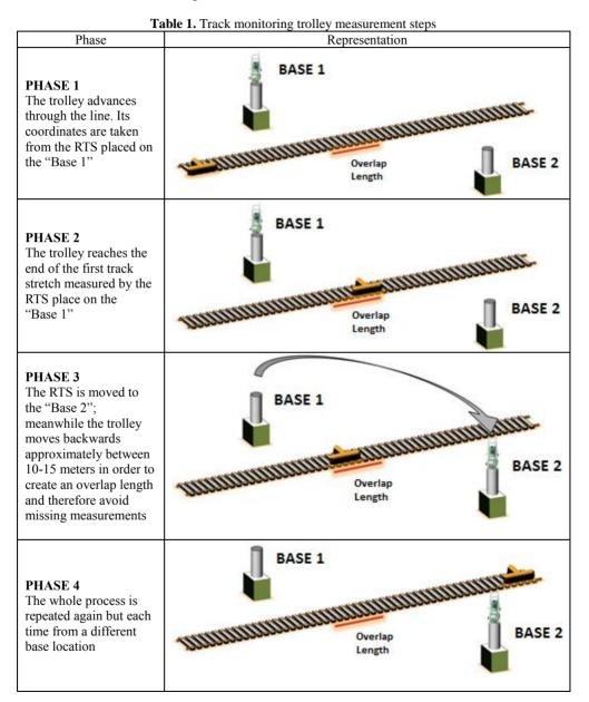
Once the measurement is done the recording data are already available. The only pretreatment that has to be made is the equally displacement representation of data, that means, obtain the data measured represented each 20 cm to be comparable with the inertial method. To obtain data equally displaced each 20 cm for both methods, an interpolation of the measurements has to be
