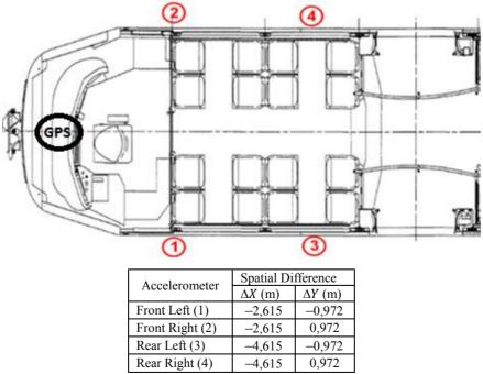
Fig. 5. Accelerometers placement and spatial differences with the GPS location
