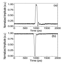
Fig. 2 (a) Electrical input pulsed signal prior to the EOM and (b) modulated optical pulse employed as pump signal.
