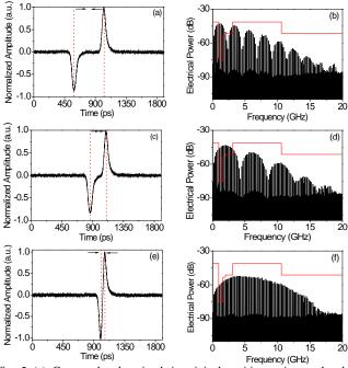
Fig. 5 (a) Generated pulses in their original position, prior to the delay configuration, (b) corresponding spectral representation, (c) generated pulses with a 200 picoseconds approximation, (d) spectral representation for the modified pulses, (e) obtained monocycle waveform after final delay configuration and (f) spectrum for the obtained UWB monocycle pulse.
