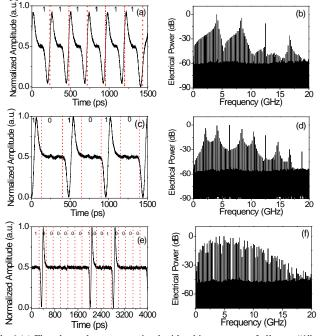
Fig.6 (a) First data scheme transmitted with a bit sequence of all ones "1" and (b) corresponding spectral representation. (c) Second data series composed of both ones "1" and zeros "0" bits and (d) respective spectrum. (e) Third data sequence transmitted and (f) electrical spectrum.
