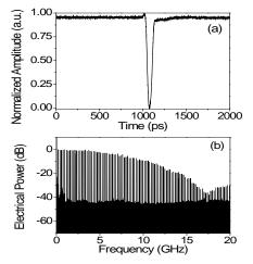
Fig. 4 (a) Negative tap pulse generated and (b) corresponding electrical spectrum.
