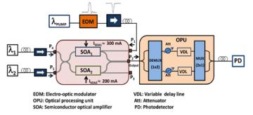
Fig.1 Experimental design for UWB signal generation and customization
