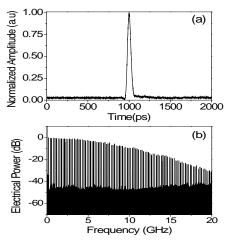
Fig. 3 (a) Positive tap pulse generated and (b) corresponding electrical spectrum.
