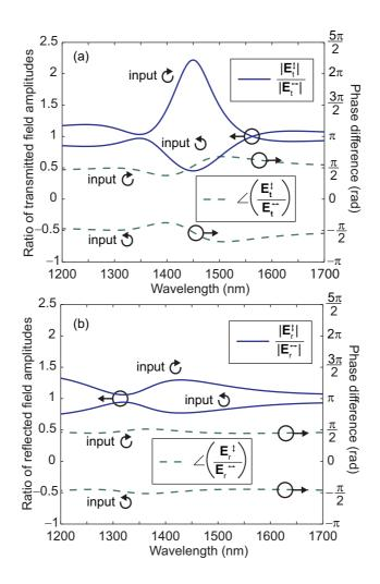
Figure 3. Effects on incident circular polarization.
