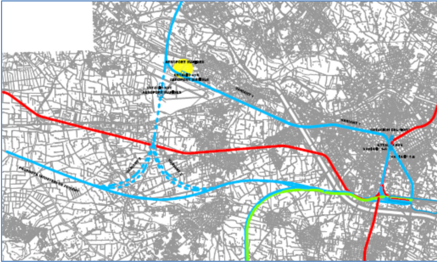
Figure 7: Study of solutions to integrate the high-speed station in Valencia City with two stations, centre and airport, 2006 (green line: in construction; blue line: high-speed planned; red line: conventional line). (Source: author.)
