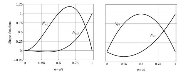
Figure 3: Left: shape functions associated to the vertical displacements  $w_1$  and  $w_2$ . Right: shape functions associated to the twist rotations  $\theta_1$  and  $\theta_2$
