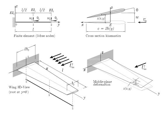
Figure 2: Geometry and 3-node finite element definition of a clamped-free wing
