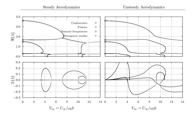
Figure 8: Frequencies ( $V\omega$  plots, top) and damping ratio (Vg plots, bottom) calculated for the 4 dof finite element model and for two aerodynamic models (steady and unsteady)
