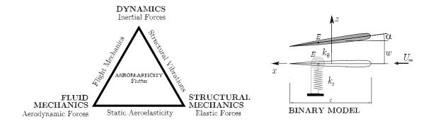
Figure 1: Left: Collar Triangle. "Aeroelasticity studies the interaction between inertial, elastic and aerodynamic forces", Arthur Collar, 1947; Right: Airfoil binary model
