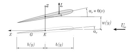
Figure 5: Rigid and elastic rotation angle of a arbitrary airfoil located at  $y = \eta l$ .
