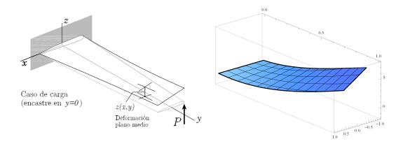
Figure 4: Elastic deformation due to a eccentric point-load at wingtip. Load case (left) and wing middle-plane deformed, calculated with Mathematica (right)
