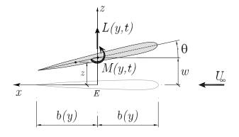
Figure 7: Lift and moment forces on the airfoil located at y coordinate
