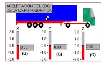
Fig, 13. Semitrailer acceleration measurement on the center of gravity.
