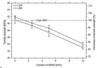
Fig. 5. Tensile strength for the blends of R5 + SEBS.
