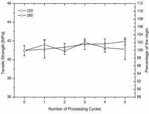
Fig. 1. Tensile strength for the reprocessed ABS.
