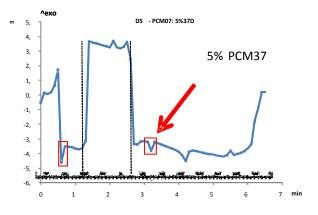
Fig. 4. DSC calorimetric curve generated by the mixture of SEBS PCM07, subjected to a heating-cooling cycle overheating.
