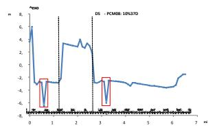
Fig. 5. DSC calorimetric curve generated by the mixture of SEBS PCM08, subjected to a heating-cooling cycle overheating.
