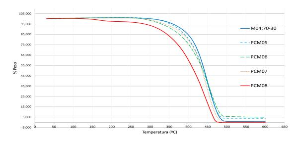
Fig. 6. Thermogravimetric comparative curves of SEBS blends (%weight vs temperature).
