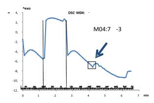
Fig. 1. DSC calorimetric curve generated by the mixture of SEBS M04:70-30, subjected to a heating-cooling cycle overheating.
