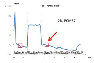
Fig. 3. DSC calorimetric curve generated by the mixture of SEBS PCM06, subjected to a heating-cooling cycle overheating.
