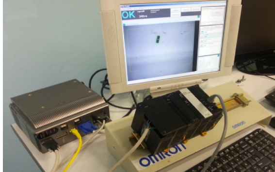
Figure 3.25: Experimental set-up: PC-based Xpectia vision system, 5 MP camera and a PLC.
