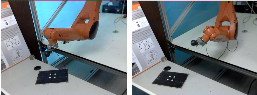
(a) Set-up for Test 1: {}^w\mathbf{M}_c(0.621, -0.101, -0.628, 1.334, 2.392, 0.626) . (b) Set-up for Test 2: {}^w\mathbf{M}_c(0.506, 0.037, -0.973, 0.861, 2.724, 0.626) .
