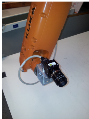
(c) 5 MP industrial camera attached to the robot end-effector.
