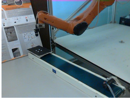
Figure 3.34: Tracking moving targets Agilus cell platform set-up.
