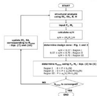
Fig. 9. Flowchart for determining continuous solution of RC column.
