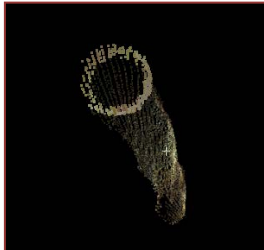
Figure 2. File A4T.xyz loaded in Cyclone for trunk center calculation.
