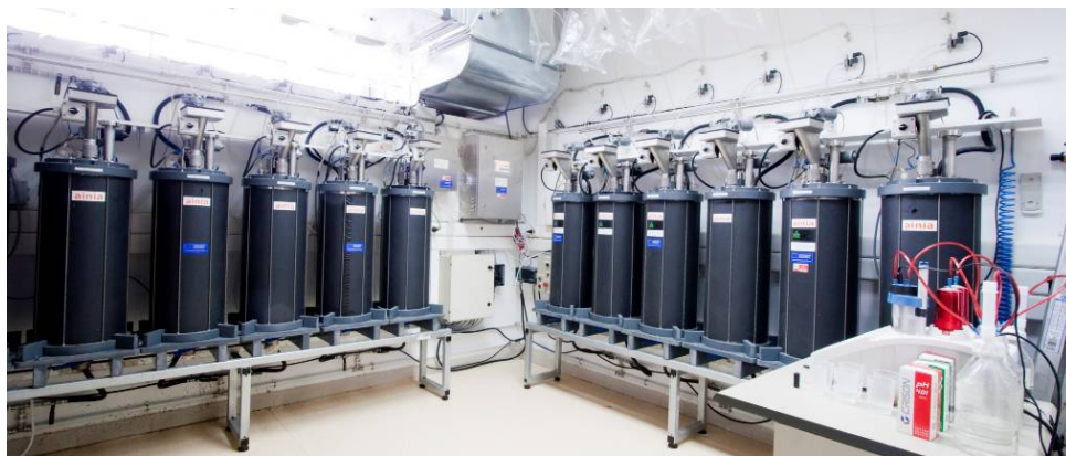
Figure 5.1. Laboratory set-up for the semi-continuous anaerobic digestion tests.
