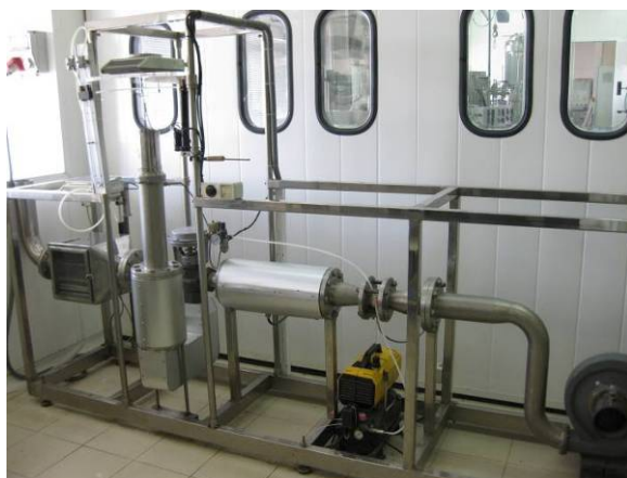
Figure 7.3. Experimental horizontal dryer used for the drying step after ethanol extraction of the orange peel.
