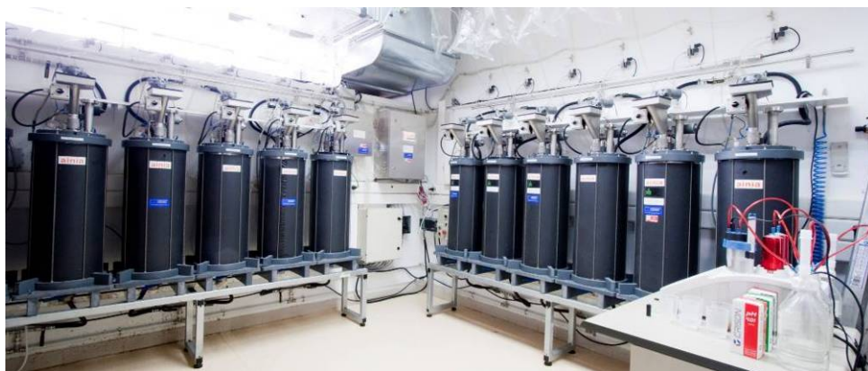
Figure 7.1. Laboratory set-up for the semi-continuous anaerobic digestion tests.
