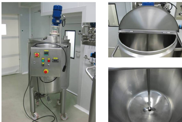
Figure 7.2. Equipment used for the ethanol extraction of the citrus essential oil from the orange peel.
