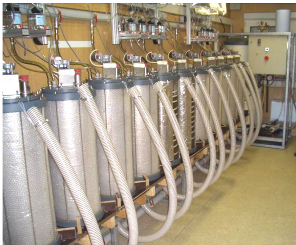
Figure 6.1. Laboratory set-up for the semi-continuous anaerobic digestion tests (LjL-ILT in Freising, Germany).
