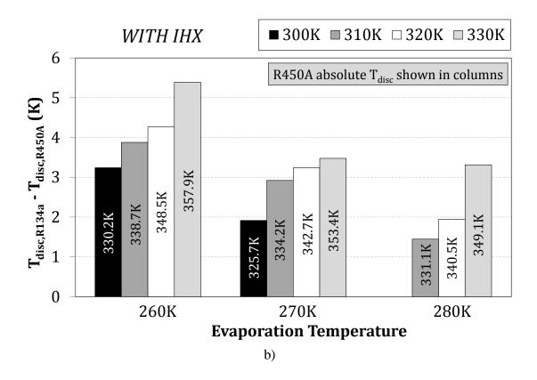
Figure 4. Discharge temperature differences between R134a and R450A a) without IHX and b) with IHX.
