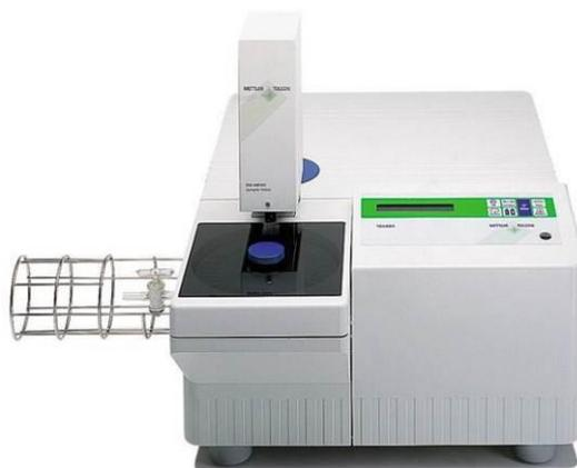
**Figura III. 2.20.-** Termobalanza Mettler-Toledo TG/SDTA 851 en EPSA-UPV
