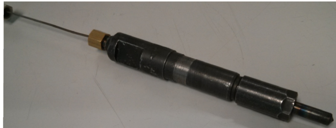
Figure 3.4. A thermocouple introduced in a modified Bosh piezoelectric injector.
