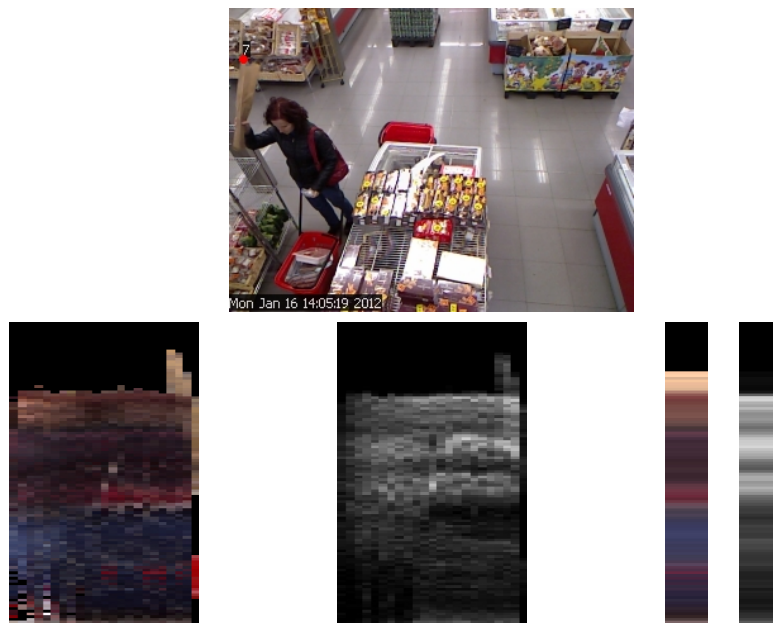
Figure 4.7: Outlier removal example. The first row shows a key frame of the person during the tracking. In the second row, from left to right: the temporal signature; the weights over time; the Bodyprint; the accumulated weight vector. The image shows a woman at the exit row of the supermarket raising a loaf of bread. The bread is segmented as part of the person. However, the accumulated weight factor indicates that its contribution in the Bodyprint is irrelevant.
