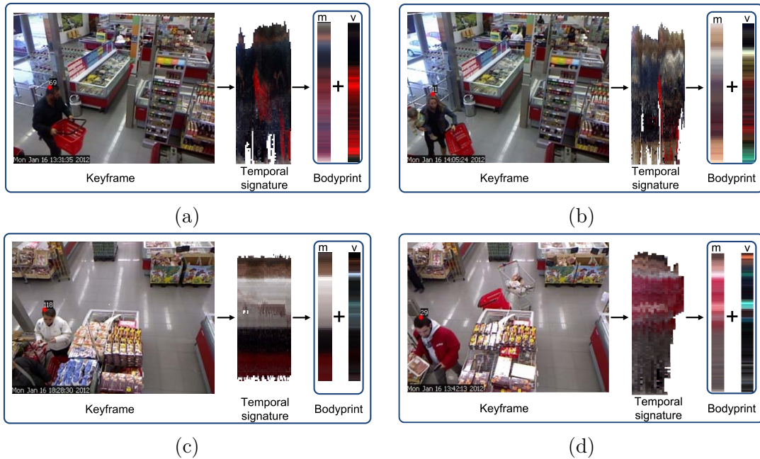
Figure 4.23: Some examples of Bodyprints and BoA descriptors with outliers generated by carried objects. In addition, figure a and c present missing data; figure a and b are strongly affected by the occlusions, where the resultant Bodyprints do not faithfully describe the appearance; figure d shows a small outlier at the person hand due to a carried object.
