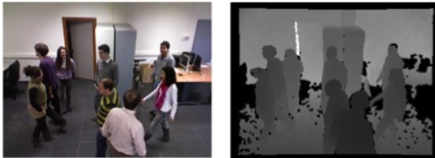
Figure 3.3: Examples of aligned RGB and depth images obtained with kinect.
