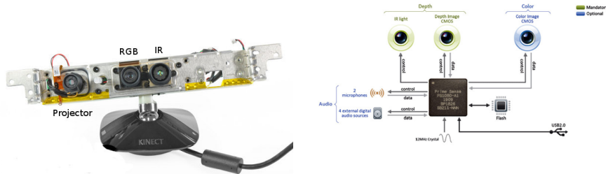
Figure 3.1: Kinect sensors: rgb camera ir camera and ir generator [Microsoft a].
