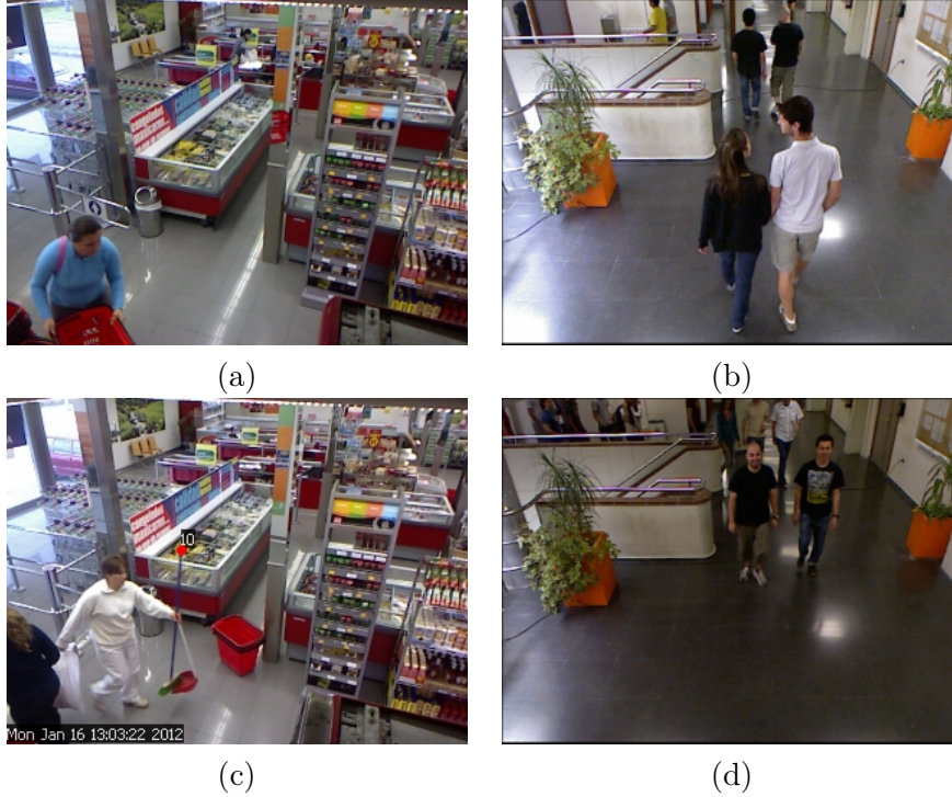
Figure 1.2: These figures show different challenging segmentations. In a) the shopping basket is difficult to be separated from the body. b) shows two people that are touching their arms, so it may not be easy to identify the edge of each silhouette. The person segmentation in c) may be difficult because of the carried bag and sweep. Finally, d) shows a man wearing a black shirt, the same color of the floor.
