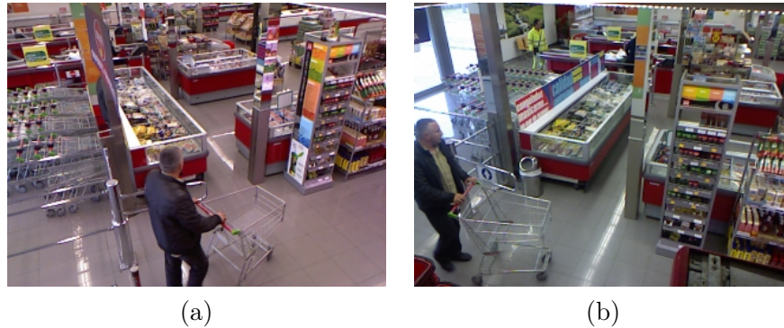
Figure 1.6: The image shows a person seen at the same instant by two different cameras located at different places. Person appearance may be totally different depending on the perspective that they are seen.
