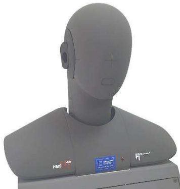
Figura 4.1: Cabeza artificial HMS III
