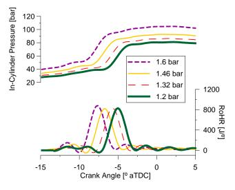
Figure 4. Instantaneous Combustion Data of Case 1 with 12% Intake Oxygen Concentration.
