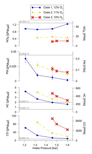
Figure 8. General Emissions for Each Test Case.
