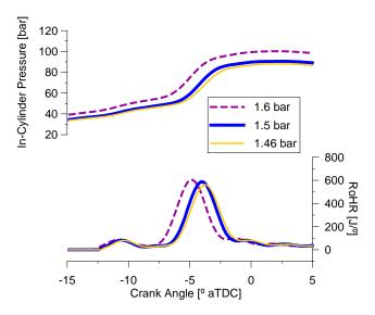
Figure 6. Instantaneous Combustion Data of Case 3 with 10% Intake Oxygen Concentration.
