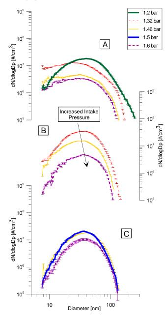
Figure 10. Particle Size Distribution Measurements for the 12% O<sub>2</sub> Case 1 (A), 11% O<sub>2</sub> Case 2 (B), and 10% O<sub>2</sub> Case 3 (C). (Particle concentrations were corrected for dilution air background particles.)
