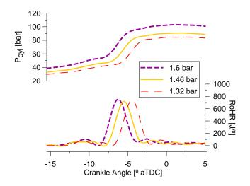
Figure 5. Instantaneous Combustion Data of Case 2 with 11% Intake Oxygen Concentration.
