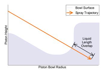
Figure 2. Fuel Spray Trajectory Relative to Piston Bowl at -24°aTDC Electronic Command Injection Timing.
