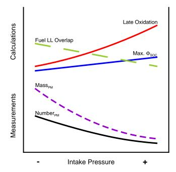
Figure 12. Visual Representation of the Effects of Intake Pressure on Premixed Diesel LTC PM Emissions.
