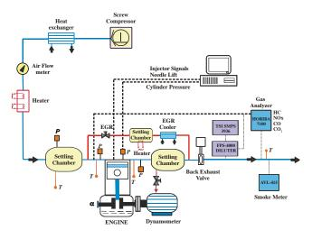
Figure 1. Design of Engine Research Laboratory.
