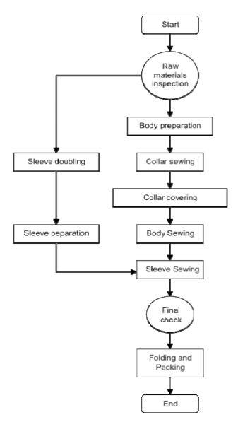
Figure 2. Process flowchart
