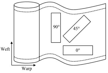
Figure 1 – Directions for cutting in the reinforcement roll.
