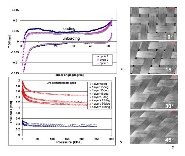
Figure 3 Fabric deformability: (a) shear diagrams: shear force *T* vs shear angle; (b) compression diagrams: fabric thickness vs. pressure (c) images of the sheared fabric;
