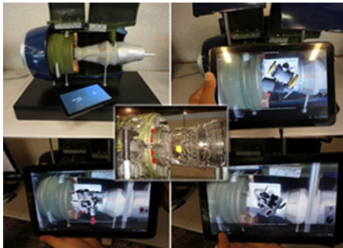
Fig. 2 Mixed reality system for troubleshooting the bleed air system.
