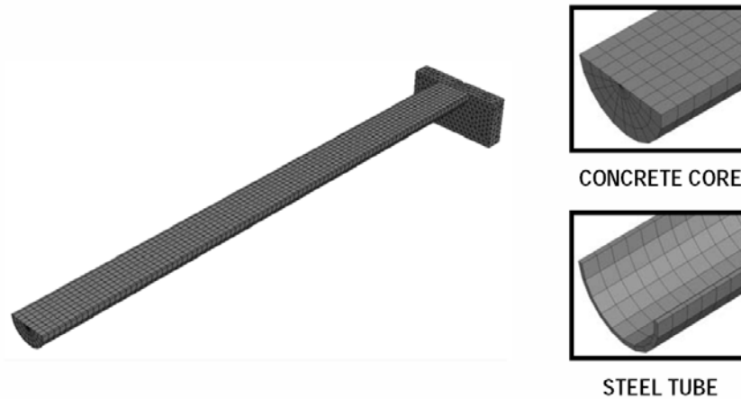
Figure 5.12. Components and finite element mesh of the three-dimensional model by Espinos et al. (2010).
