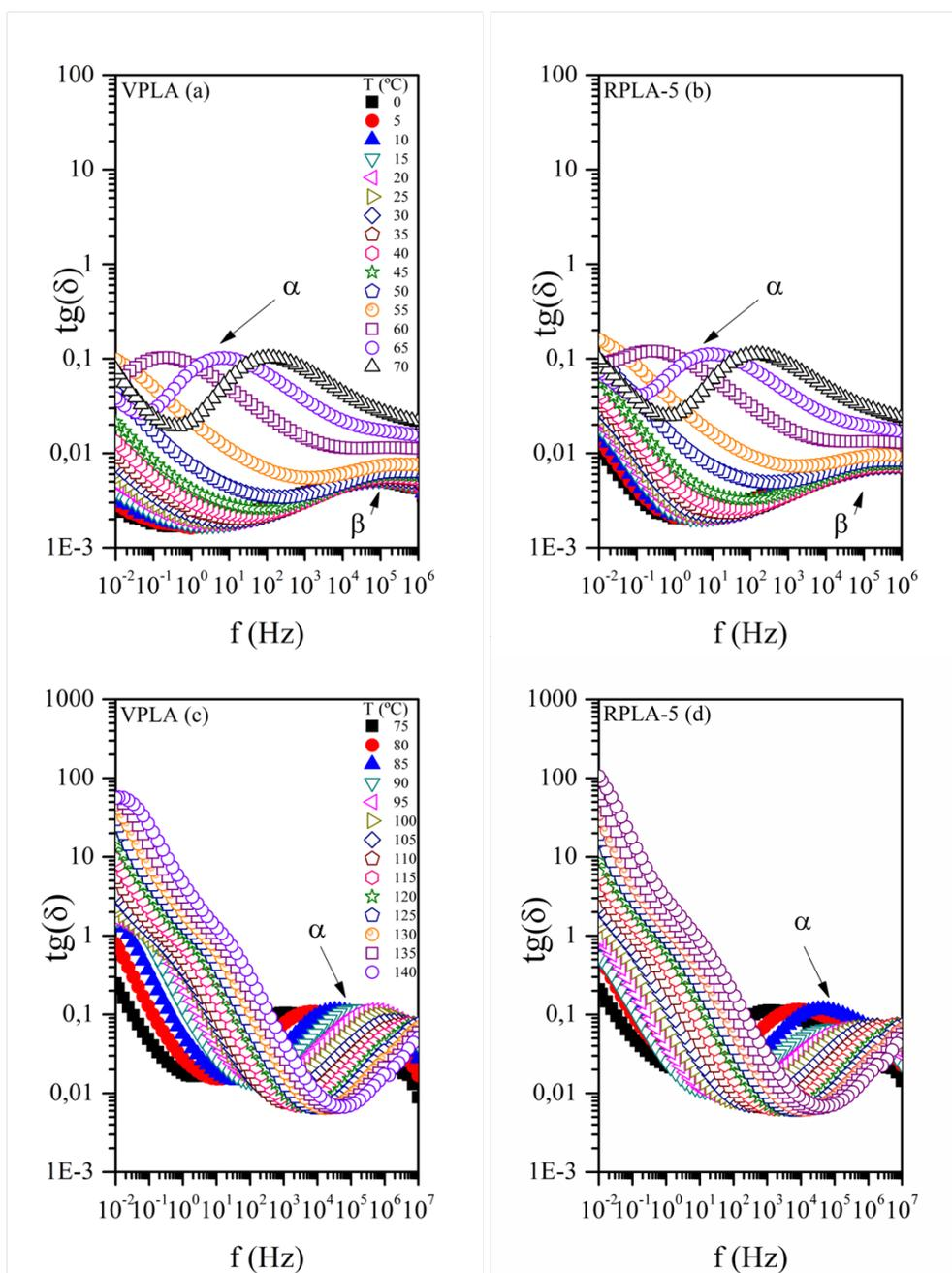
**Figure 3.** Isotherms showing the frequency response of virgin polylactide VPLA (left) and PLA reprocessed 5 times RPLA-5 (right) at temperatures range of ( $0^{\circ}\text{C} \leq T \leq 70^{\circ}\text{C}$ ) (up) and ( $75^{\circ}\text{C} \leq T \leq 140^{\circ}\text{C}$ ) (down) in terms of loss tangent,  $tg(\delta)$ .
