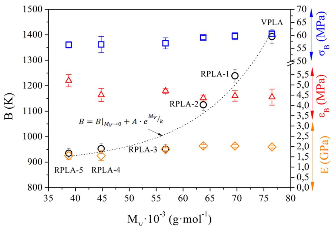
**Figure 5.** Exponential correlation of the fragility parameter  $B$  with the decay of molar mass due to thermo-mechanical degradation. Comparison with macromolecular mechanical properties: stress at break  $\sigma_B$ , strain at break  $\epsilon_B$  and elastic modulus  $E$ .
