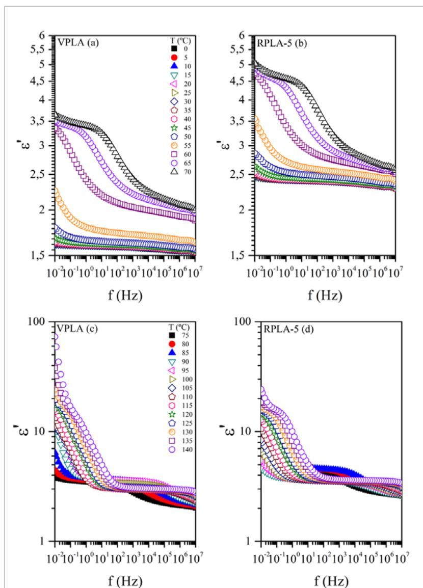
**Figure 1.** Isotherms showing the frequency response of virgin polylactide VPLA (left) and PLA reprocessed 5 times RPLA-5 (right) at temperatures range of ( $0^{\circ}\text{C} \leq T \leq 70^{\circ}\text{C}$ ) (up) and ( $75^{\circ}\text{C} \leq T \leq 140^{\circ}\text{C}$ ) (down) in terms of real component of the dielectric permittivity,  $\epsilon'$ .
