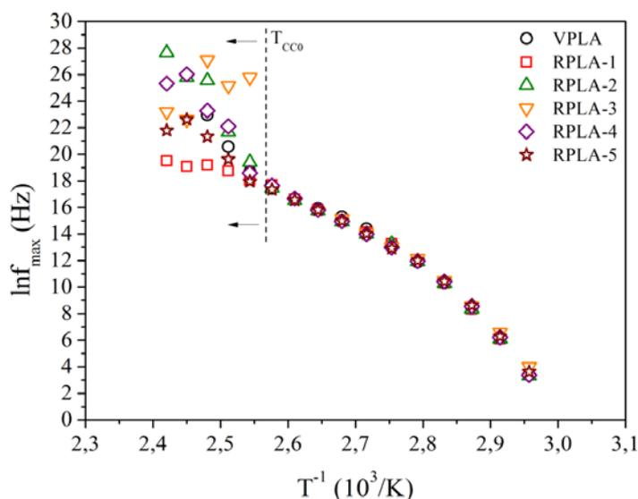
**Figure 4.** Arrhenius maps of the  $\alpha$  relaxations corresponding to virgin and recycled poly(lactides) (VPLA and RPLA-i). Deviation from VTFH model at temperatures higher than the cold-crystallization is remarked.
