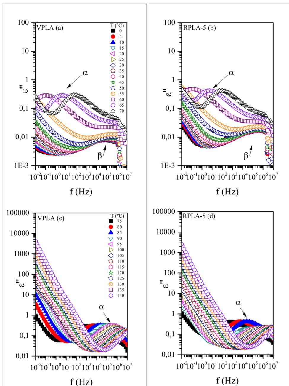
**Figure 2.** Isotherms showing the frequency response of virgin polylactide VPLA (left) and PLA reprocessed 5 times RPLA-5 (right) at temperatures range of ( $0^{\circ}\text{C} \leq T \leq 70^{\circ}\text{C}$ ) (up) and ( $75^{\circ}\text{C} \leq T \leq 140^{\circ}\text{C}$ ) (down) in terms of imaginary component of the dielectric permittivity,  $\epsilon''$ .
