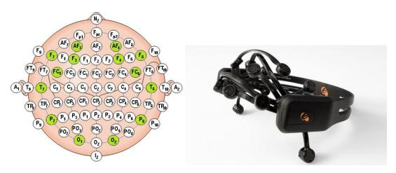
Figure 1. A) Emotiv EPOC electrode positioning. B) Emotiv EPOC device.
