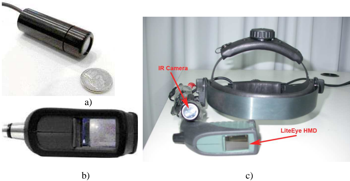
Figure 1. a) The IR bullet camera used b) The LiteEye-500 monocular OST HMD. c) Capture and visualization system (IR camera and the LiteEye HMD)
