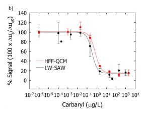
Fig. 2. (a) Immunoassay cycle; (b) LM-SAW and HFF-QCM standard calibration curves for carbaryl determination
