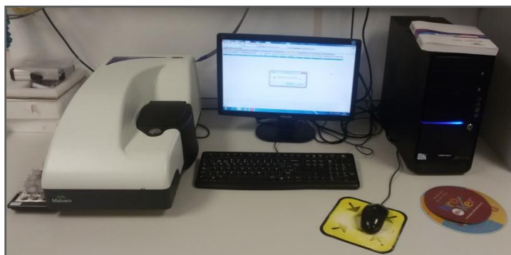
Figura VI.9: Zetasizer Nano ZS90.
