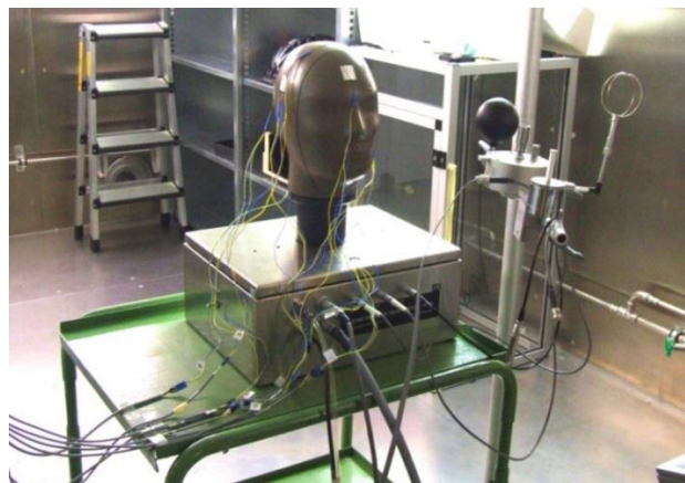
Figure 2.6. Laboratory setup for head manikin temperature calibration.
