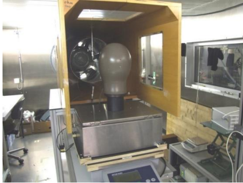
Figure 2.2. Standard setup for thermal testing of headgear including wind effect.
