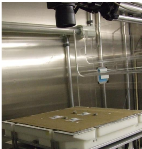
Figure 4.6. Experimental setup for measuring attached sensors effect on dry and wet heat transfer experiments.
