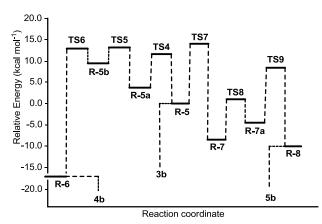
Fig. 3 B3LYP/6-31G\*\* Energy profiles for the radical transformations of 3b leading to 4b and 5b in benzene; 3b, 4b and 5b are off the scale.
