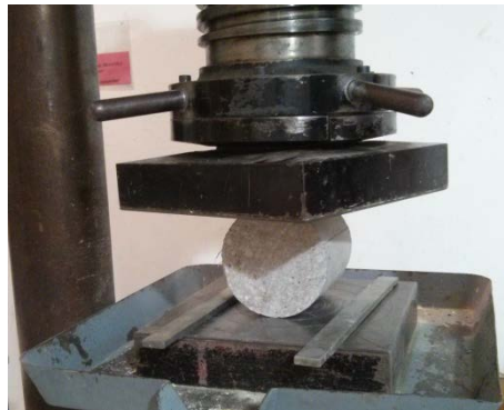
Figure 1 - Pre-cracking process of a concrete specimen
