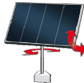
Figure 6. Two axis tracker (elevation / azimuthal) [4]
