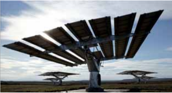
Figure 7. ADES™ two axis monopost tracker (Photovoltaic)
