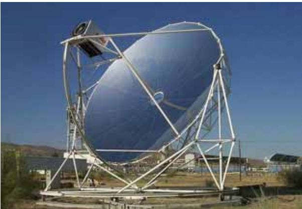
Figure 8. SBP™ two axis tracker (Concentrator)
