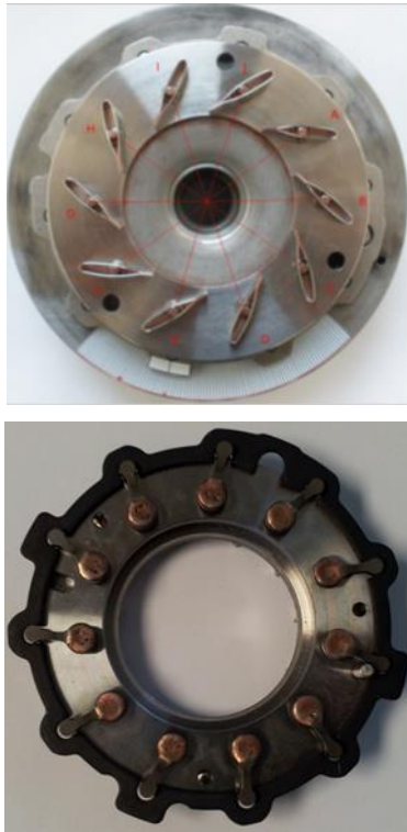
Fig. 1 Photo of stator vanes in fully open position. The reference radial direction is indicated for each vane.
