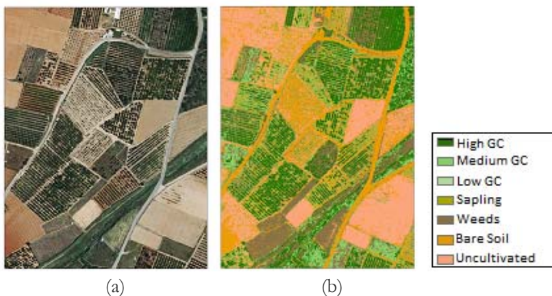
Figure 1. Reflected solar radiation in the visible RGB (a) and the thematic map of training areas (b).
