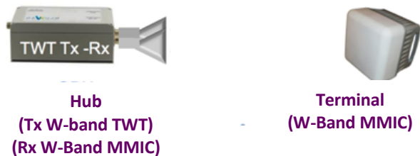
Figure 1. Transceiver concept (ODU Outdoor Unit)
