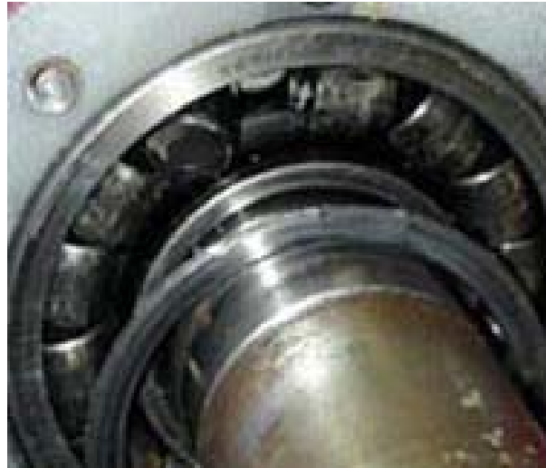
Fig. 12. Image of the motor with bearing failure.
