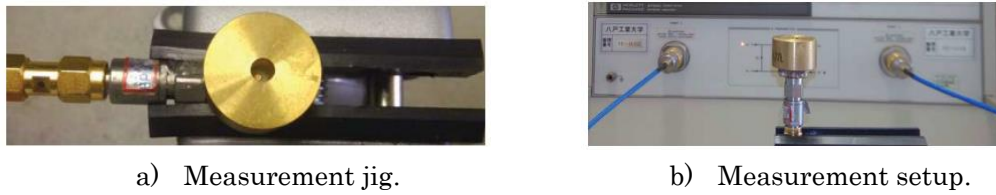
Figure 1.5. Open-ended coaxial line reflection method presented in [5].
