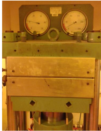
Figure 7. Uniaxial press machine for lamination process
