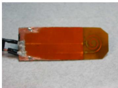
a) Close-up of spiral sensor
