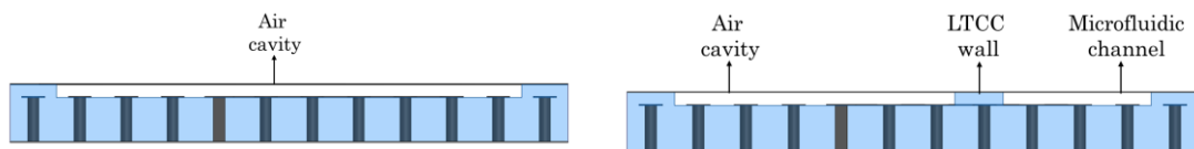
Figure 5.5. Front view of the gap waveguide resonator: Without and with the LTCC wall to separate the air cavity from the microfluidic channel.
